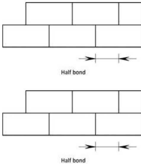
In practice, to maintain proper bonding, the cutting of masonry units to avoid straight joints is unavoidable; however, if the building is designed to standard masonry modules and correctly set out, the cutting of masonry units can be kept to a minimum.
